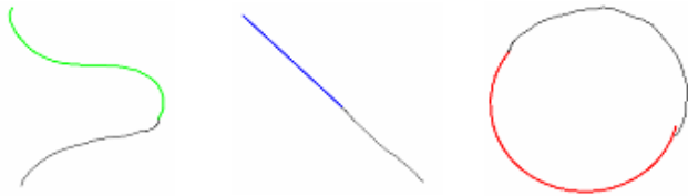
Figure 1. Examples of continuation strokes (shown in black; previously recognized shapes shown in color); current systems will recognize the continuation strokes as separate primitives rather than combining the stroke with a previously drawn stroke.
